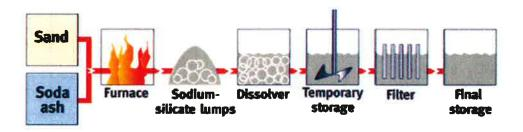
b) Solutions of soluble silicates ("waterglass") may be produced either by dissolving the soluble silicate lumps in water at elevated temperatures (and partly at elevated pressure) or for certain qualities also by hydrothermally dissolving a reactive silica source (mainly silica sand) in the respective alkali hydroxide solution according to the equation:
